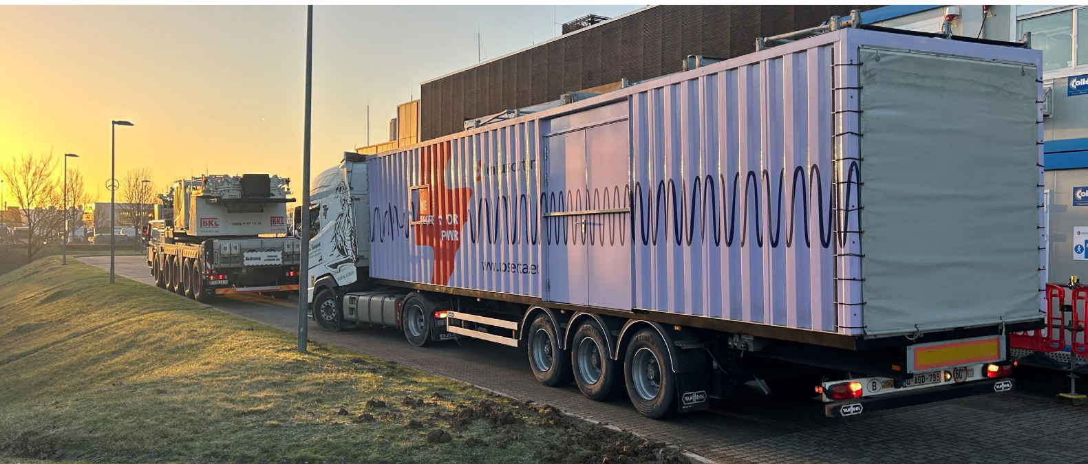
(Foto 8 - 1600 kVA mobiele UPS Luminus Solutions)
